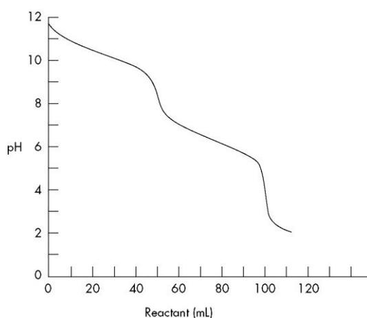
The titration curve of this acid–base reaction was measured by taking continuous readings from a pH electrode in the conical flask. Solution A (0.1 M, 50 mL) was placed in a conical flask and titrated against 0.1 M solution B.
